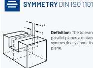
**Definition:** The tolerance zone is limited by two parallel planes a distance t apart and disposed symmetrically about the datum axis or datum median plane.
