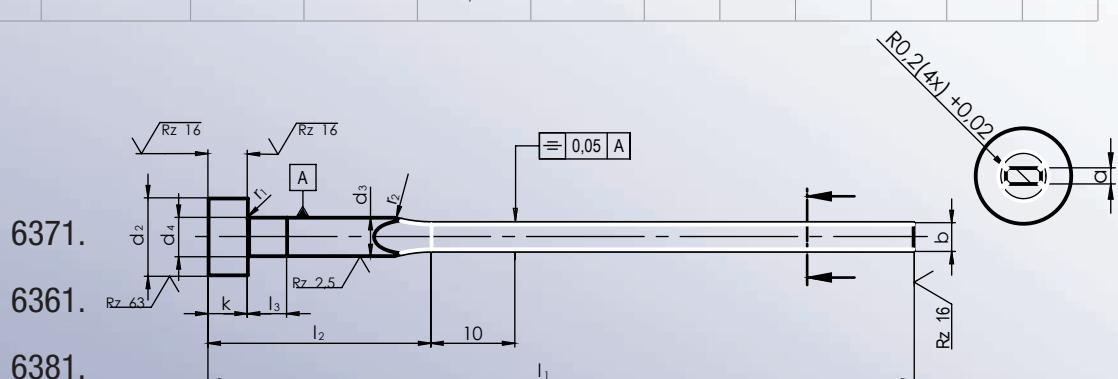
» Version: Head warm compressed - shaft highly tempered and hardened, finally polished
